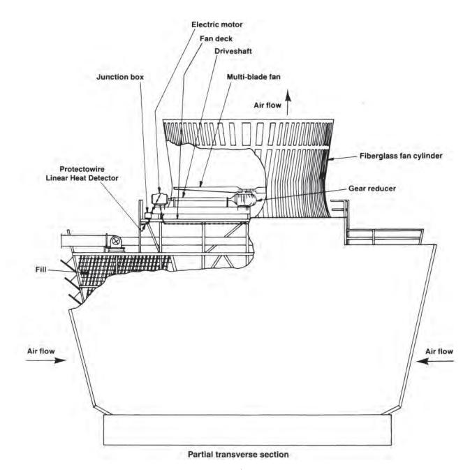
Protectowire Linear Heat Detector is illustrated in a cross-flow cooling tower. Copper wire is run in conduit from the fire alarm control panel to the junction box mounted on the fan deck flooring. From this point the Detector is looped over the fan motor, circled around the inside perimeter of the fan cylinder base just beneath the fan deck and returned to the junction box.
