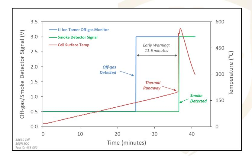
Li-ion Tamer® detects off-gas <u>prior</u> to thermal runaway
