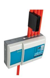
ECO reliably detects unseen hazards by conditioning or filtering the air to remove moisture, interferent<sup>\*</sup> gases, dirt and other particulates that can cause traditional point gas detection systems to false alarm or become contaminated.
